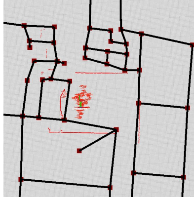
(a) The prior map (in this case extracted from a crude line drawing) is shown with black lines (corners as brown squares). The current live sensor data (2D lidar) is shown with red points. The particle cloud, used in a Monte Carlo localisation implementation that localizes the sensor data against the prior map, is shown as red arrows.
